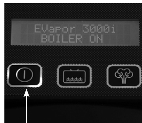
Switch on the unit by pressing the main switch (3) Now the boiler is turned on and the machine will pump water into the boiler.
