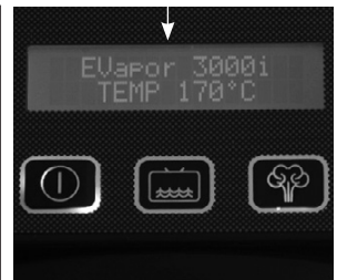
The machine needs about 8-10 minutes to convert the water into dry vapor. Once it reaches operating pressure, this appears on the display (4).and the display signals that it is ready for use.
